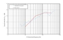
The overall performance of our enclosure depends on a lot of variables such as weight, size, panel types, ventilation, hatches, cable penetrations etc. It is therefore impossible to give an exact air-borne noise reduction value without at least some of the variables known. Indicative values can be given after an initial informative discussion.
